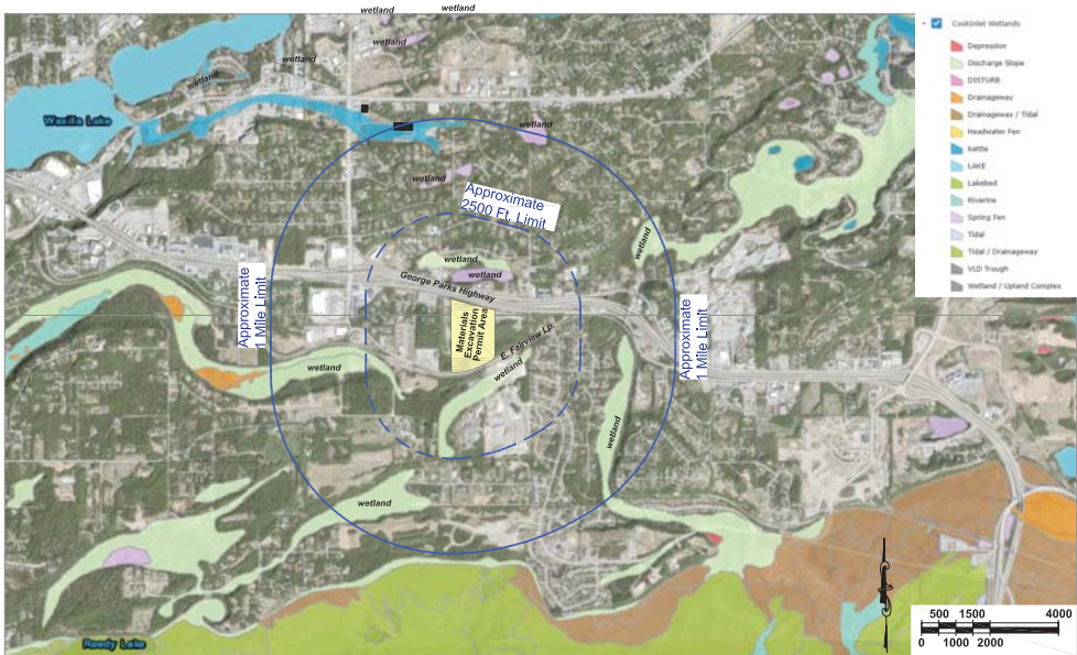
SWPPP Map B General Location Map with Wetlands and Water Bodies within 1 Mile and 2500 Feet of the Project Amendment 2, 9-18-24
