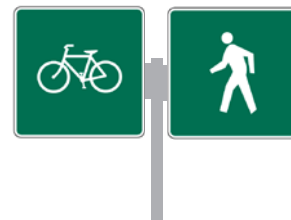
Figure 4-21. MUTCD signing options for specifying user types and path positioning can be used to indicate which users belong on the separate parts of a separated bike lane corridor (D11-1a, D11-2).
