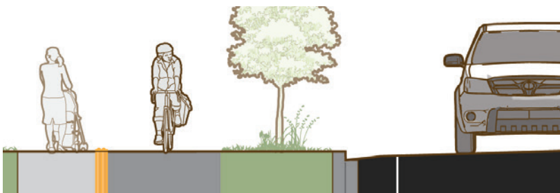
Figure 4-20. Separation from the sidewalk is valuable for reducing unwanted pedestrian encroachment into the bike lane. The use of physical separation with vertical elements, unpaved separation, or detectable edges may be more effective than visual delineation.
