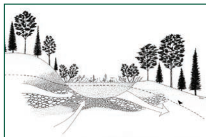
This diagram depicts shallow groundwater flowing through relatively permeable sediments into and out of a wetland.
