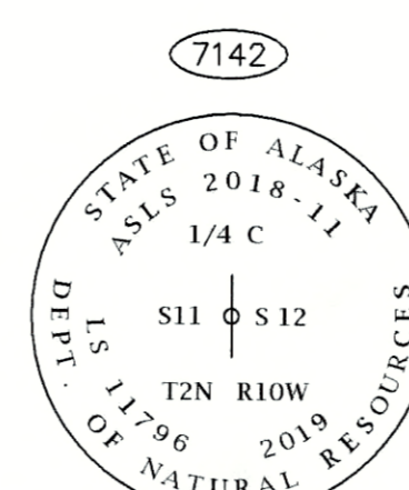
Found 3-1/4" Aluminum Cap On a 30" x 2-1/2" Aluminum Flare End Post 0.2' AGL; Carsonite Post 1' North < 4" Spruce B.T. bears N32°E, 33.6' < 9" Spruce B.T. bears S82°E, 50.2' < 6" Spruce B.T. bears S53°W, 50.5'
