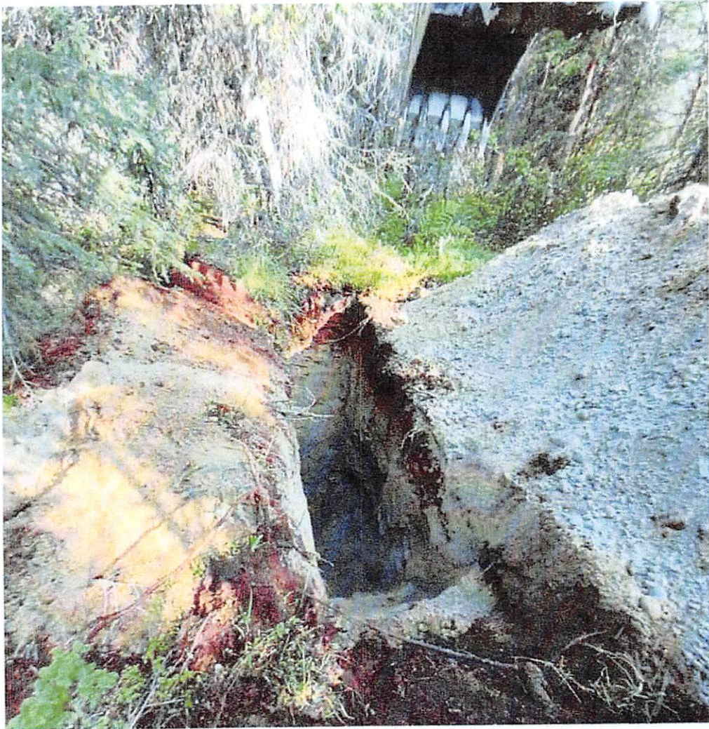
Test Pit Lot 2 - 16', no water, impervious layer
