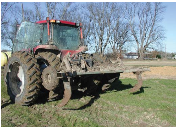
Figure 5. A mechanical sub-soiler.
