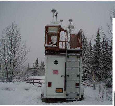
Size selective inlet for PM<sub>10</sub> and Very sharp cut cyclone for PM<sub>2.5</sub>
